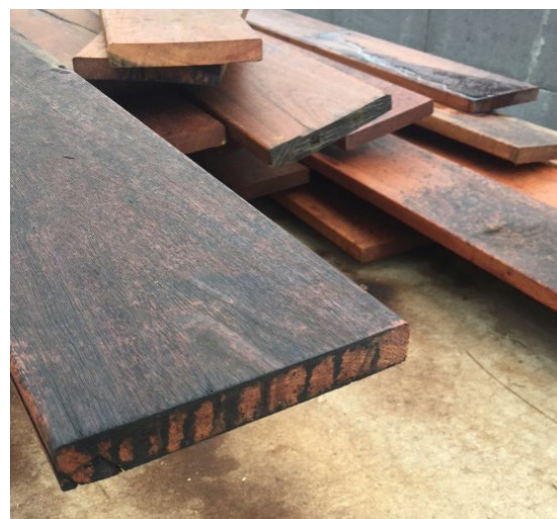
Photograph 2 - Mould stains on linseed oiled decking
